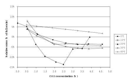
Figure 3. Valtronics CO2 sensor (Mod. 2015); temperature effects in dry gas. Relative errors (expressed as per cent of full scale) vs. CO<sub>2</sub> concentrations. Each solid line represents one temperature.
