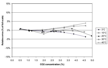
Figure 2. Texas Instruments CO<sub>2</sub> sensor (TI9GS-4); temperature effects in dry gas. Relative errors (expressed as per cent of full scale) vs. CO<sub>2</sub> concentrations. Each solid line represents one temperature.
